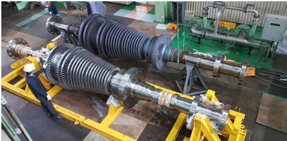
New Rotor (Bottom) and Old Rotor (Top) Prior to Installation
