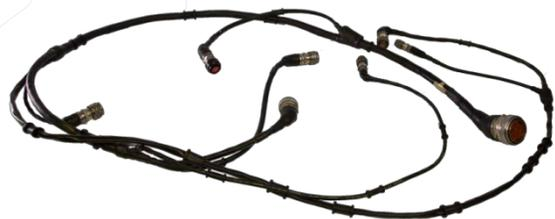
**CASE STUDY****CFM56 Thermocouple and Wiring Harness
